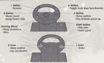
If you're using an Interact<sup>®</sup> Steering Wheel with a D-pad, you can use the D-pad to move the menu cursor. Also, while in the game, press the D-pad ↑ to toggle the Track Map/Speedometer Press ↓ to reverse.
